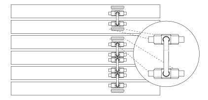
NOTE: Install the SCSI cable by carefully pressing the cable connector against the StackMaster<sup>TM</sup> TX12 connector until the connectors snap into place.
